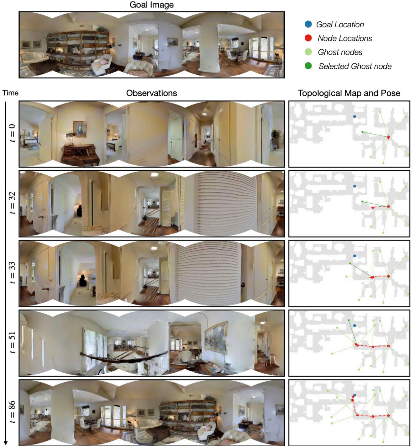
Figure 9: Example Trajectory Visualization. Figure showing a visualization of an example trajectory using the NTS model. Agent observations are shown on the left and the topological map and pose are shown on the right. Note that the map and the goal location are shown only for visualization and are not available to the NTS model. ( t=0 ) NTS model creates the first node and adds the ghost nodes. Note that ghost node locations are not predicted, the model predicts only the direction of ghost nodes. The model correctly selects the correct ghost node closest to the goal. ( t=33 ) The NTS model creates the second regular node and adds ghost nodes. Note that the ghost node in the direction of the second node from the first node are removed. ( t=51 ) The NTS model creates another new node. ( t=86 ) The agent reaches the goal after creating 4 nodes as shown in the trajectory on the map and decides to take the stop action.
